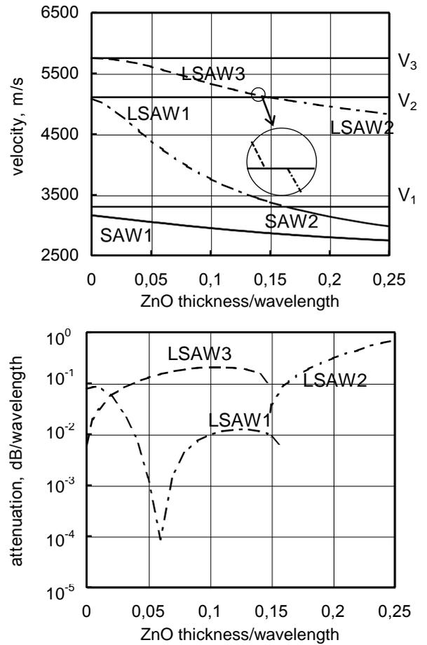
Fig. 1. Propagation characteristics of SAWs and LSAWs in ST,X cut of quartz as functions of normalized ZnO thickness.  $V_1$ ,  $V_2$  and  $V_3$  are the limiting velocities of bulk waves
