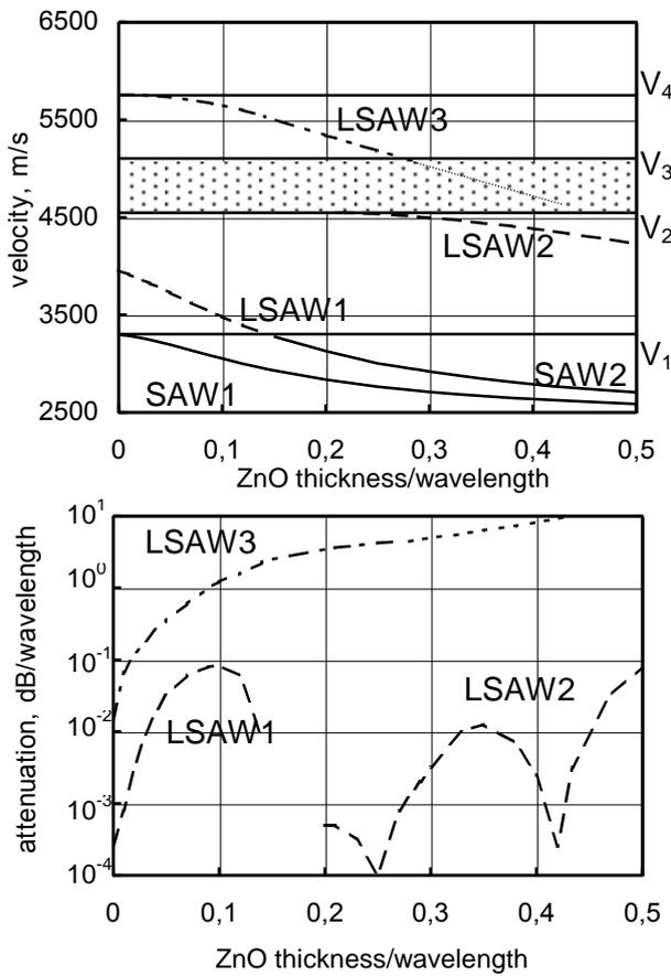
Fig. 4. Propagation characteristics of SAWs and LSAWs on metallized surface of LST cut of quartz with ZnO overlay as functions of ZnO thickness.
