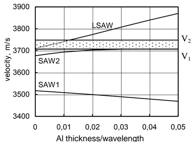
Fig. 6. Velocities of SAWs and LSAW on metallized surface of LBO, Euler angles (45°, 90°, 70°) with aluminum overlay, as functions of overlay thickness
