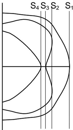
Fig. 3. Slowness section in the sagittal plane of LST cut of quartz.
