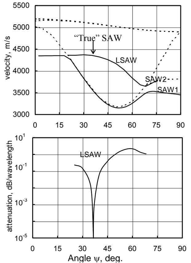
Fig. 5. Propagation characteristics of SAWs and LSAWs on metallized surface of LBO, Euler angles (45°, 90°,  $\psi$ ). Dotted lines show the limiting velocities.
