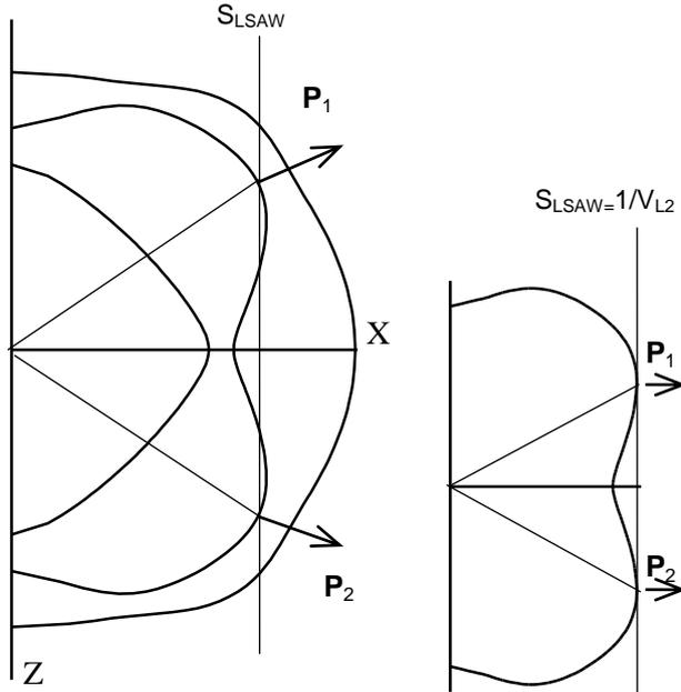
Fig.5. Slowness section in quartz, Euler angles  $(0^\circ, 50^\circ, 0^\circ)$ , with simple reflection solution for fast quasishear mode. In the fragment this solution degenerates into CEW.
