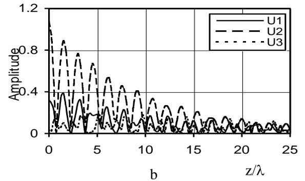
Fig.6. Displacement components versus depth for LSAWs propagating in quartz, Euler angles  $(0^\circ, 50^\circ, 25.14^\circ)$  (a) and  $(0^\circ, 50^\circ, 25.0^\circ)$  (b).
