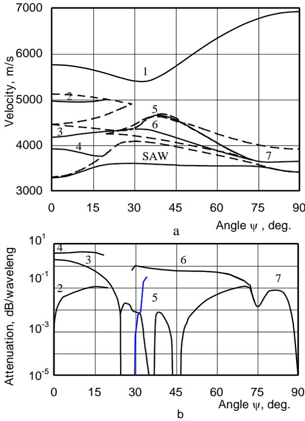
Fig.1. Velocities (a) and attenuation coefficients (b) of SAW, leaky solutions (solid lines) and limiting bulk waves (dashed lines) in quartz cuts ( $0^\circ$ ,  $50^\circ$ ,  $\psi$ ) versus angle  $\psi$ .
