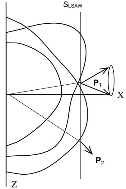
Fig.4. Slowness section in quartz, Euler angles ( $0^\circ, 50^\circ, 47^\circ$ ). The cone of Poynting vectors  $\mathbf{P}_1$  corresponds to degenerate quasishear bulk waves.
