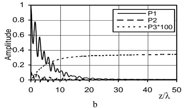
Fig.7. Poynting vector components versus depth for LSAWs propagating in quartz, Euler angles  $(0^\circ, 50^\circ, 25.14^\circ)$  (a) and  $(0^\circ, 50^\circ, 25.0^\circ)$  (b).
