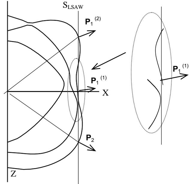
Fig.2. Cross-section of the slowness surface by the sagittal plane in quartz cut with Euler angles ( $0^\circ$ ,  $50^\circ$ ,  $30^\circ$ ). Poynting vectors  $\mathbf{P}_1$  (two variants) and  $\mathbf{P}_2$  refer to two contributing partial bulk waves when the propagation velocity of leaky wave is  $V_{LSAW}$ .
