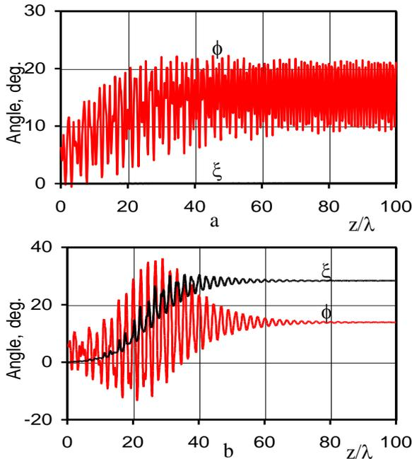
Fig.8. Azimuth  $\phi$  and declination  $\xi$  angles of Poynting vector versus depth for LSAWs propagating in quartz, Euler angles  $(0^\circ, 50^\circ, 25.14^\circ)$  (a) and  $(0^\circ, 50^\circ, 25.0^\circ)$  (b).
