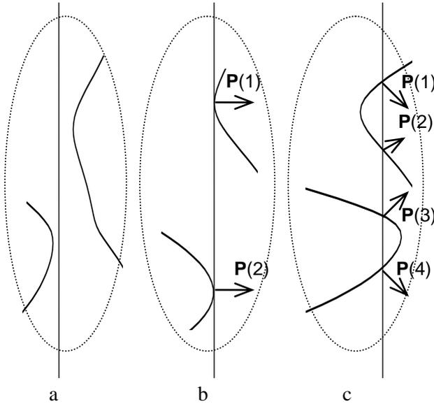
Fig.3. Fragments of slowness sections when there is a concavity for slow quasishear branch. Leaky solution includes (a) none of two bulk waves, (b) two limiting waves, (c) incoming and outgoing bulk waves.
