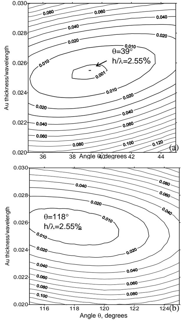
Fig.3. Contour plots of attenuation coefficients ( $\text{dB}/\lambda$ ) of HVPSAW propagating in  $\text{LiTaO}_3$ , Euler angles ( $0^\circ, \theta, 90^\circ$ ), with **periodic gold grating**, versus Euler angle  $\theta$  and normalized film thickness: a)  $\theta=25\text{-}35^\circ$ ; b)  $\theta=115\text{-}125^\circ$ .
