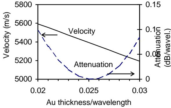
Fig.6. Propagation velocity and attenuation at resonance frequency in LT orientation with Euler angles ( $0^\circ, 39^\circ, 90^\circ$ ), versus normalized thickness of Au grating.
