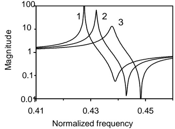
Fig.7. Amplitude of strip admittance  $Y$  versus normalized frequency  $f' = fp/v_{BAW}$ , in three LT orientations ( $0^\circ, \theta, 90^\circ$ ) with optimized thickness of Au grating: 1 -  $\theta=39^\circ$ ,  $h/\lambda=2.55\%$ , 2 -  $\theta=34^\circ$ ,  $h/\lambda=2.4\%$ , 3 -  $\theta=28.5^\circ$ ,  $h/\lambda=2.25\%$ ,
