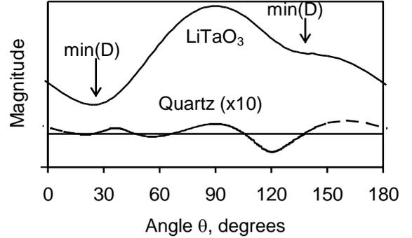
Fig.1. Determinant of mechanical boundary conditions  $D$  calculated for the quasi-longitudinal SSBW propagating in orientations of  $\text{LiTaO}_3$  and quartz with Euler angles  $(0^\circ, \theta, 90^\circ)$ .
