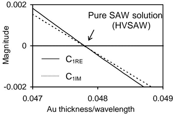
Fig.4. Real and imaginary parts of coefficient  $C_1$  illustrating contribution of quasi-shear bulk partial wave into HVPSAW solution in LT cut ( $0^\circ; 29^\circ; 90^\circ$ ) with uniform Au film, versus film thickness.
