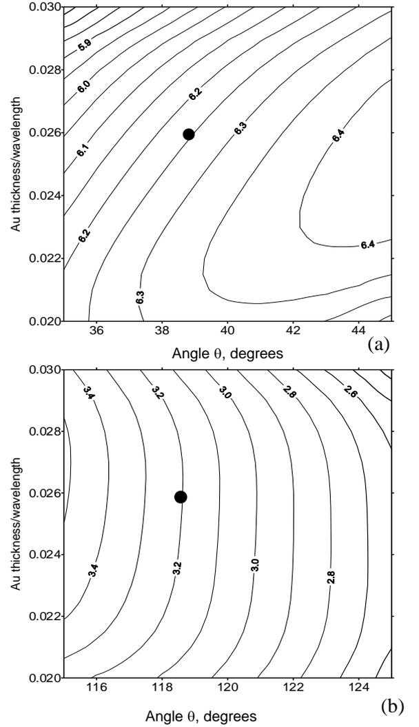
Fig.5. Contour plots of electromechanical coupling coefficient  $k^2$  (%) of HVPSAW propagating in  $\text{LiTaO}_3$ , Euler angles ( $0^\circ; \theta, 90^\circ$ ), with **periodic gold grating**, versus Euler angle  $\theta$  and normalized film thickness: a)  $\theta=35-45^\circ$ ; b)  $\theta=115-125^\circ$ . The sign “•” marks the optimal angle  $\theta$  and thickness, providing minimum propagation loss, according to Fig.4.
