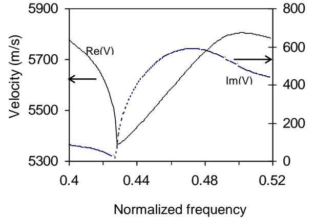
Fig.8. Velocity dispersion of HVPSAW propagating in  $\text{LiTaO}_3$ , Euler angles ( $0^\circ, 39^\circ, 90^\circ$ ), with Au grating  $h/\lambda=2.55\%$ , versus normalized frequency.
