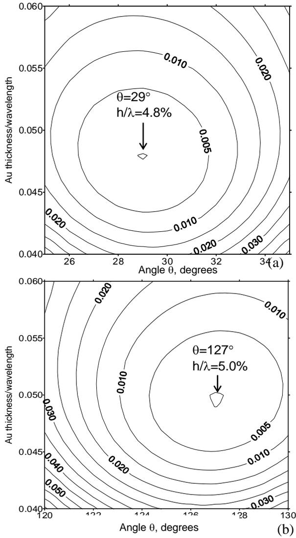
Fig.2. Contour plots of attenuation coefficients ( $\text{dB}/\lambda$ ) of HVPSAW propagating in  $\text{LiTaO}_3$ , Euler angles ( $0^\circ, \theta, 90^\circ$ ), with **uniform gold film**, versus Euler angle  $\theta$  and normalized film thickness: a)  $\theta=25\text{-}35^\circ$ ; b)  $\theta=120\text{-}130^\circ$ .
