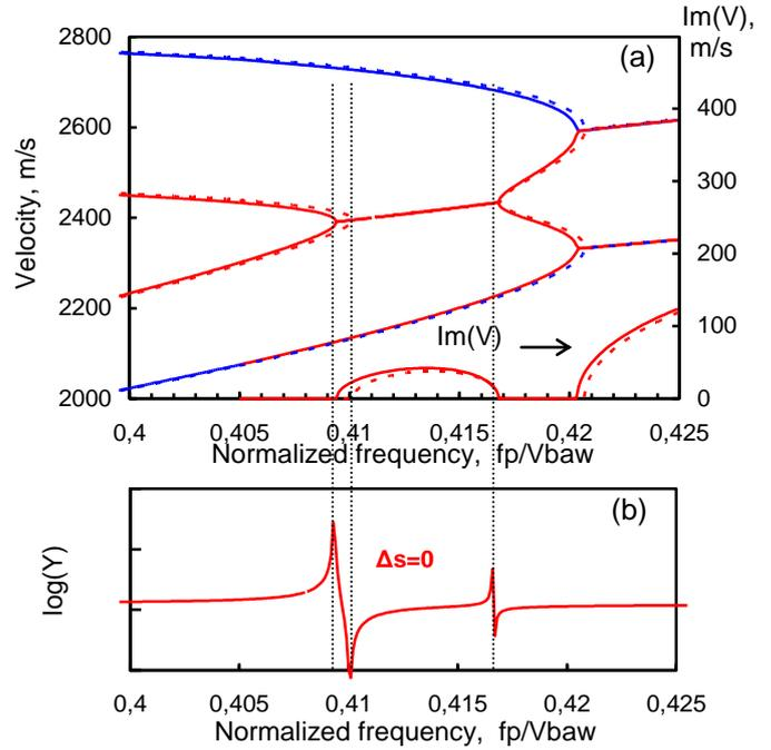
Fig.6. Velocity dispersion in SC and OC gratings (a) and harmonic admittance calculated at synchronous resonance condition (b), in Pt grating on LGS, when electrode thickness is  $h=4\%\lambda$
