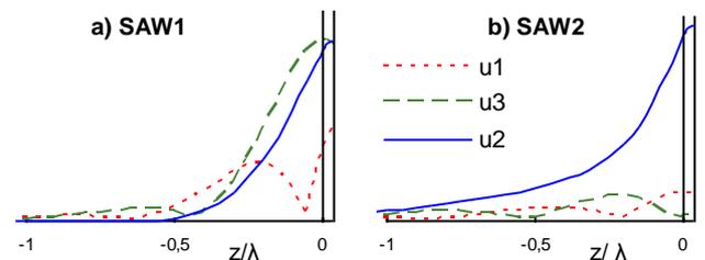
Fig.9. Displacements along vertical axis, in LGS with Pt grating (SC),  $h_{\text{pt}}=4\% \lambda$ , calculated at normalized frequency  $f'=0.4$ : (a) SAW1, (b) SAW2.
