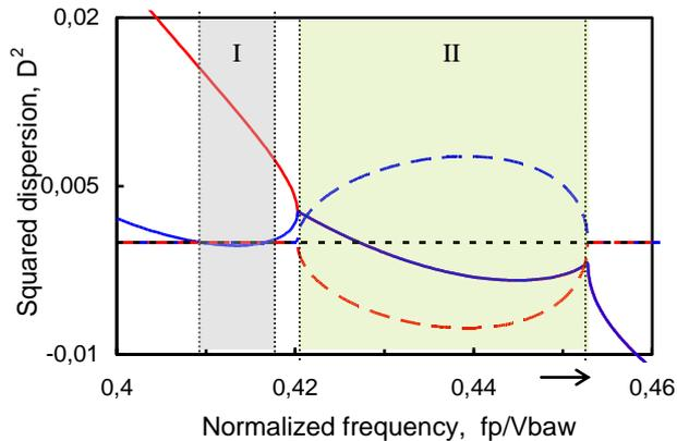
Fig.7. Real (solid lines) and imaginary (dashed lines) parts of dispersion parameter  $D^2=(\Delta s/s_0)^2$ , as functions of normalized frequency, in SC grating with Pt electrodes on LGS,  $h=4\% \lambda$ . Two stopbands refer to interactions between counter propagating SAW1 (shaded area I) and counter propagating SAW1 and SAW2 (area II).
