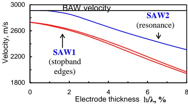
Fig.2. Velocities of two SAW modes propagating in LGS with Pt grating estimated at resonant frequencies, as functions of normalized electrode thickness
