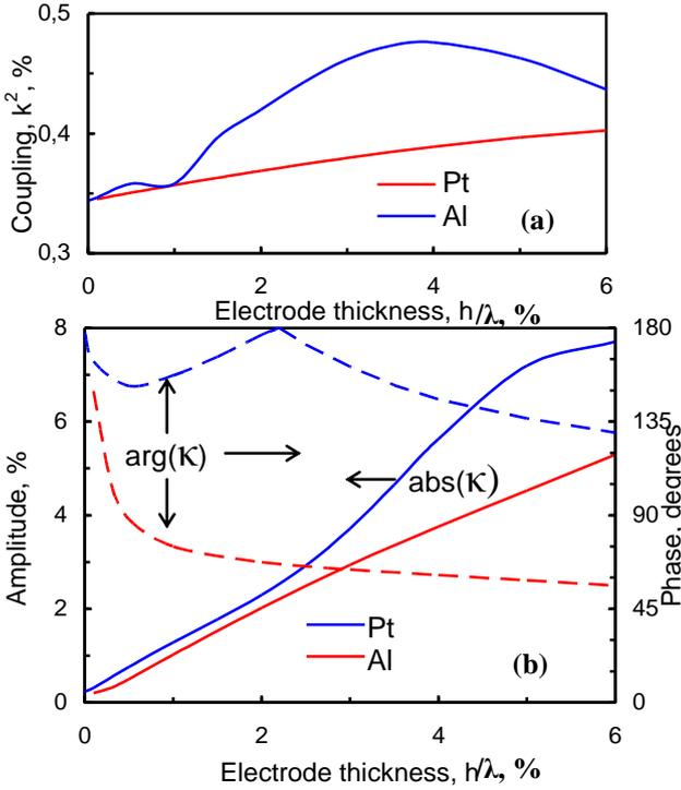
Fig.1. Characteristics of SAW in LGS with Pt grating, as functions of electrode thickness: electromechanical coupling (a) and reflection coefficient per wavelength (b). The module and phase of reflection coefficient for Pt grating (blue lines) are compared with that of Al grating (red lines).
