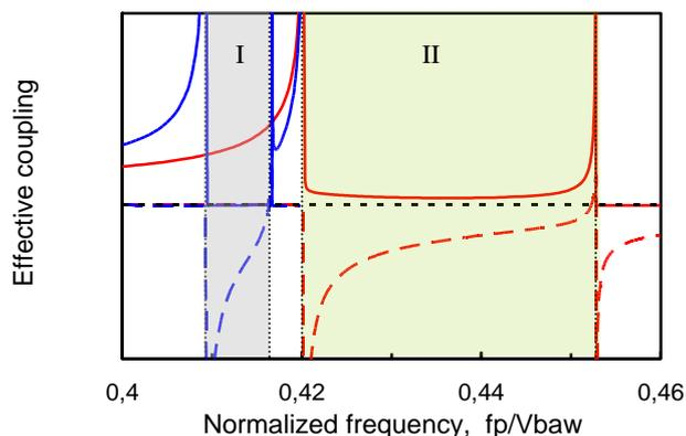
Fig.8. Real (solid lines) and imaginary (dashed lines) parts of effective coupling coefficient  $K_{\text{eff}}$ , as functions of normalized frequency, in SC grating with Pt electrodes on LGS,  $h=4\% \lambda$ .
