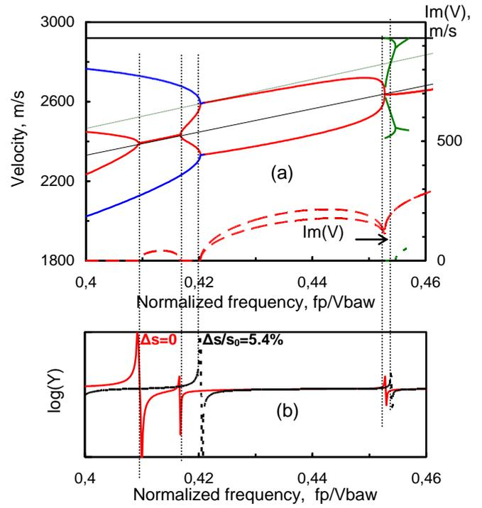
Fig.5. Velocity dispersion in SC grating (a) and harmonic admittance calculated at  $\lambda=2p$  and at certain detuning (b), in Pt grating on LGS, when electrode thickness is  $h=4\%\lambda$
