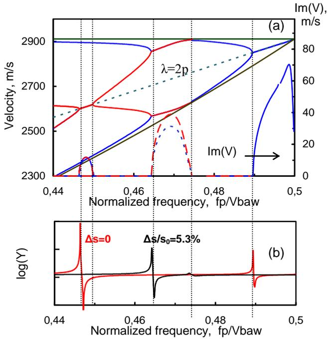
Fig.4. Velocity dispersion in SC grating (a) and harmonic admittance calculated at synchronous resonance (b),  $\lambda=2p$  and at certain detuning, in Pt grating on LGS, when electrode thickness is  $h=2\%\lambda$
