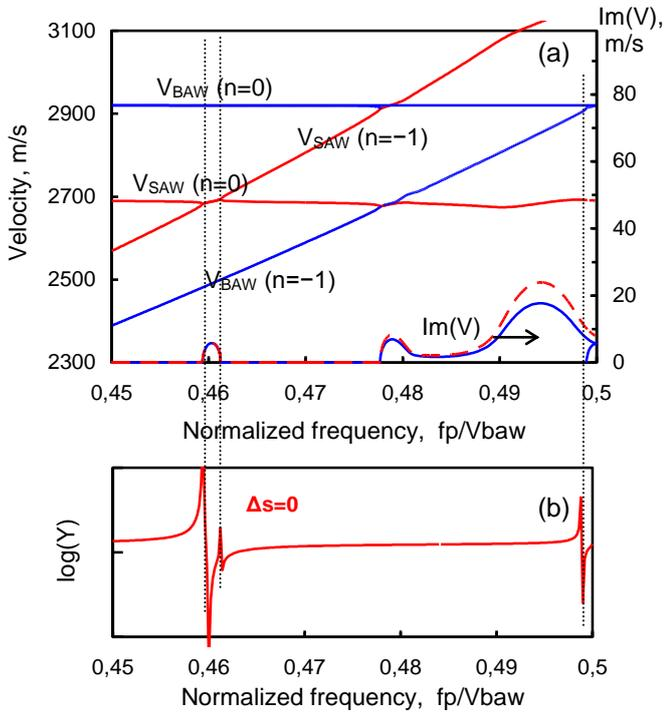
Fig.3. Velocity dispersion in SC grating (a) and harmonic admittance calculated at synchronous resonance condition (b), in Pt grating on LGS, when electrode thickness is  $h=1\%\lambda$
